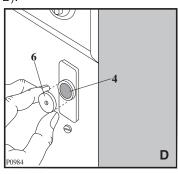
If the door has to be opened from left to right, invert the position of the plates (7), the magnet (4) and the plate (5) (Fig. B and E). Mount the counter-magnet (6) and the hinges (1) as previously described.
